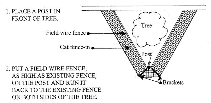
NOTE: THE FENCING MATERIAL CAN BE PURCHASED AT ANY LOCAL HARDWARE STORE. IT HAS A 2 X 4 INCH WIRE MESH AND IS CALLED BY MANY NAMES SUCH AS "FIELD WIRE," "WELD WIRE," "DEER FENCE," ETC.
